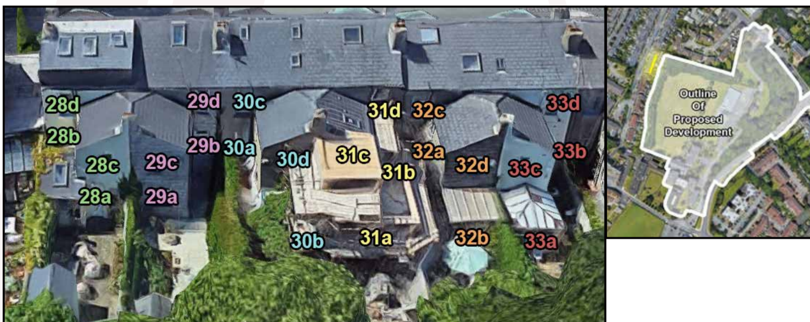
Figure 5.15: Left & Centre - Highlighted areas indicate the position of assessed windows., Right - Aerial view of assessed location
